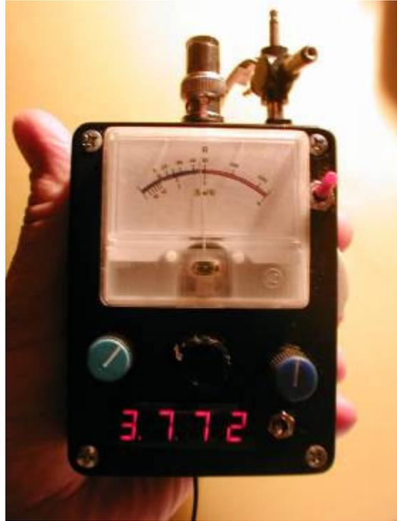
The completed “Mk1” antenna analyser
